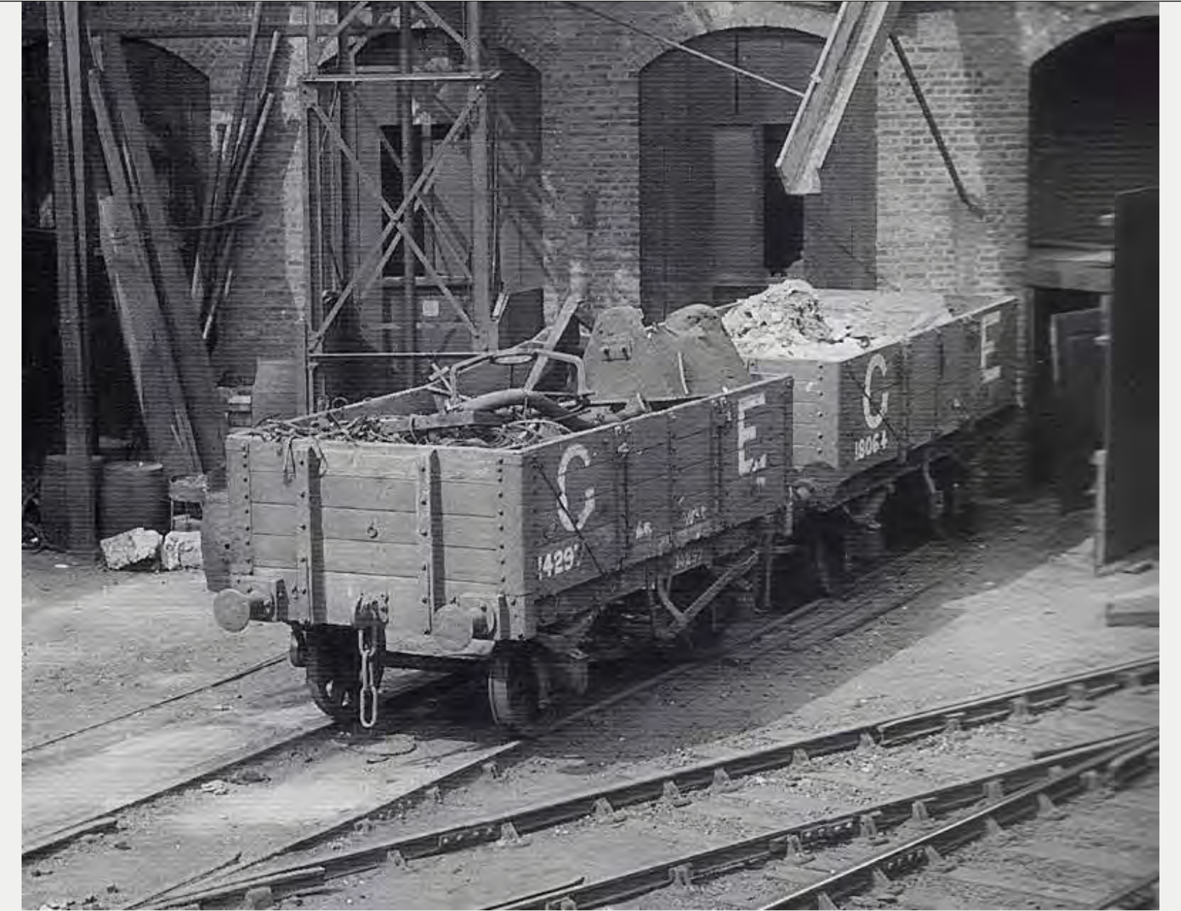
ARCHIVE IMAGE OF THE LIGHT BAR: 'TWO GONDOLAS AT THE NORTON FOLGATE POWER STATION OF GER, LOADED WITH SCRAP. PROBABLY TAKEN AROUND 1903.'
